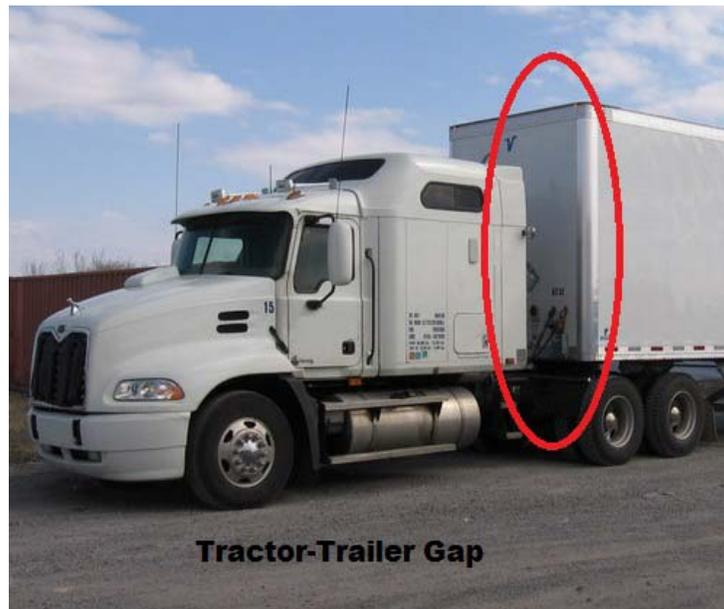
Figure 13 – Typical tractor-trailer gap
