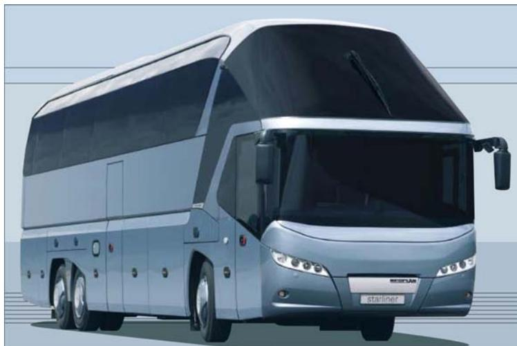
Figure 22 – German-designed intercity bus with  $C_D \approx 0.35$ .
