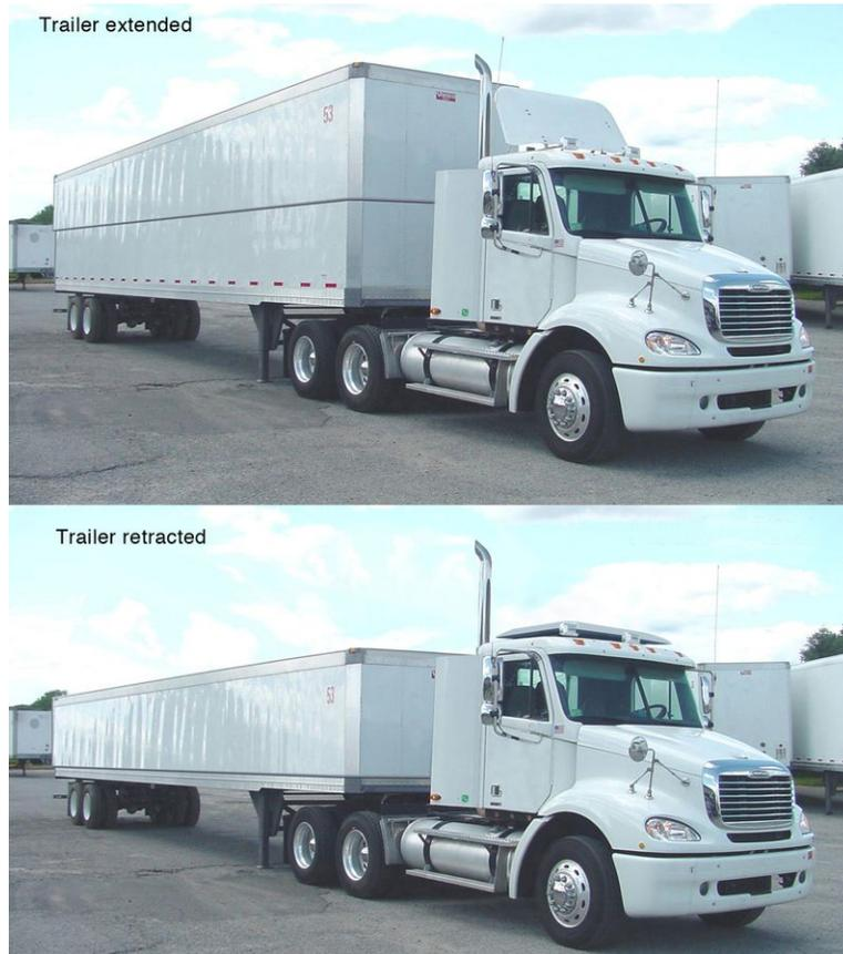
**Figure 20 – Retractable trailer concept**
