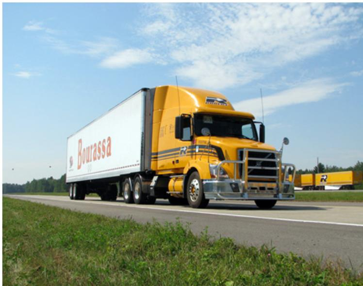
**Figure 10 – Heavy duty bumper mounted to a tractor**
