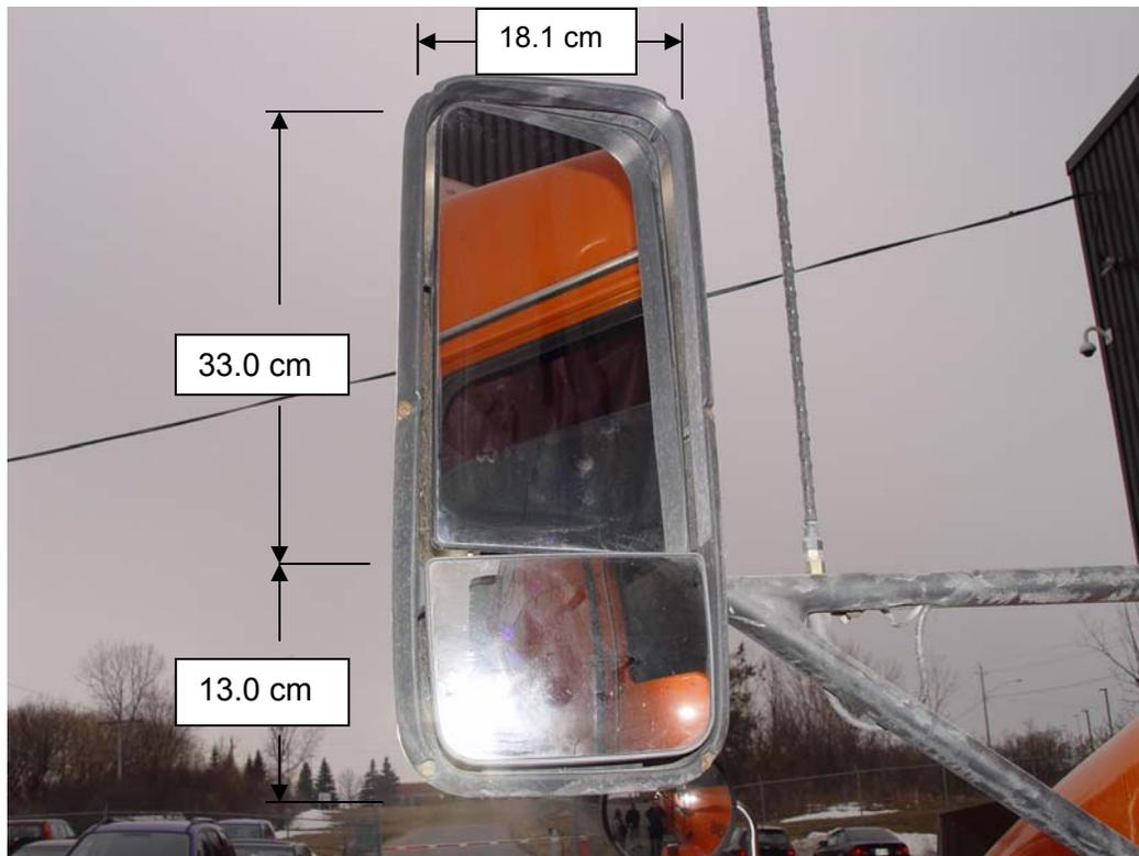
Figure 8 – View of typical driver's side mirror
