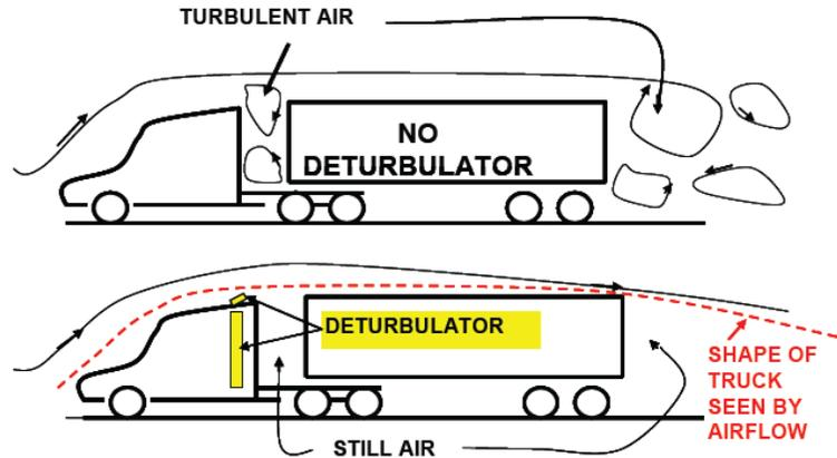
Figure 11 – Effect of deturbulator on a tractor trailer [95]
