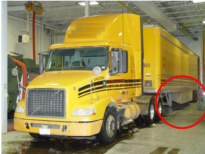
Figure 17 – Example of typical side skirt
