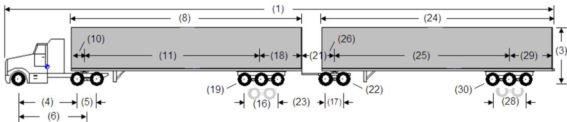
Figure 1 – Illustration of a long combination vehicle (LCV) [16]
